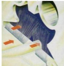
The unique intermediate cooling curtain design sprays mist like coolant onto the air that has been compressed in the first stage, rapidly reducing the temperature.
